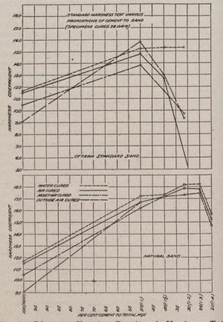
Fig. 1.—Diagram Showing Results of Hardness Tests of Cement Mortars.
