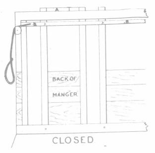
ple, durable, and has given good satisfaction, and is as seen in the following diagrams. It will close from one to twenty cows by pulling on the rope, and they may be liberated by raising (Fig. A.), so that the stanchion may pass back under it. All the movable uprights are joined together by two strips under the top of the bales, and parallel with it, one on each side
