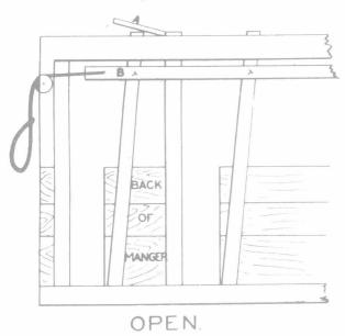
of the uprights, and are fastened together by putting a block between and held with a bolt, as seen in Fig. B. Each of the uprights are joined to this by an iron pin, with a keyhole in it, and a leather key placed therein to keep it from working out. This pin may be taken out if one cow is desired to be let out, and if all but one the pin may be removed and a block placed behind the upright to hold it closed. A. DERRICK.
