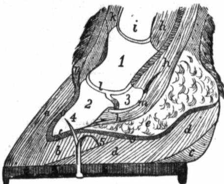
This drawing was taken from a hoof to show the result of a cold rolled and sheared pointed nail, which produced the death of a valuable animal, and for which carelessness the owner received no remuneration.
