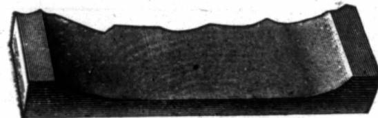
This drawing represents a cross section of iron from which the cold punched and sheared nails are made by forcing a blank therefrom by means of a punch
