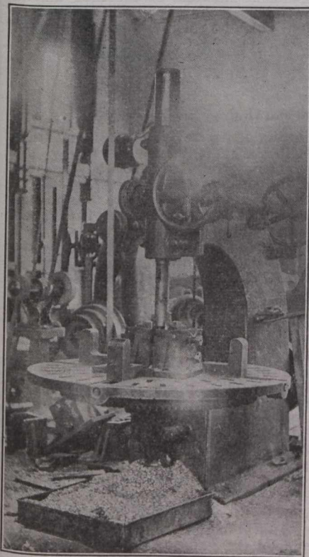
Old Vertical Boring Mill used for Boring Journal Brasses.
