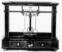
FOUR-INCH BEAM BUTTON BALANCE. The most important improvement is in the base which is extended on either side so as to include the pan-rest
