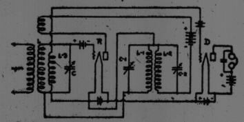
may be used, these coils being shunted by the variable condensers (C-1) and (C-2) each having a capacity of 0.001 macrofarad. These condensers have a comparatively large capacity due to the necessity of providing a bypass for the high frequency oscillations which otherwise would be choked by the high inductive effect of the coils (L-1) and (L-2). These coils should be supported on a coll mounting so that the proper inductive relation may be obtained by varying the coupling.
