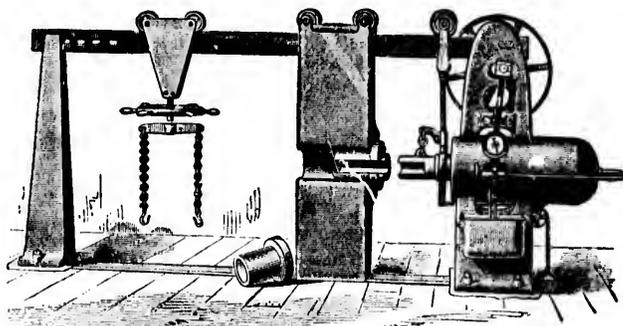
THE SELLERS HYDROSTATIC WHEEL-PRESS, IN MACHINERY HALL.
