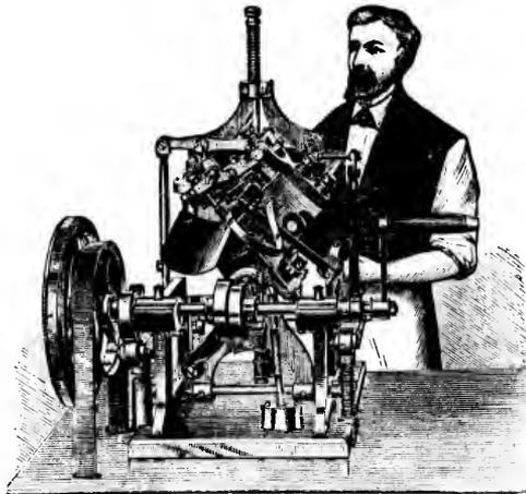
JOHNSON'S TYPE CASTING MACHINE, IN MACHINERY HALL.
