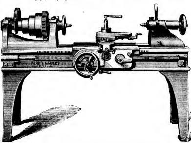
SCREW-CUTTING LATHE, EXHIBITED IN MACHINERY HALL.
