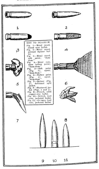
Figure 1 is a full-size drawing of a metal cased, thirty calibre, round nose bullet, as used in a military rifle. Thirty calibre signifies that the diameter of the bore of the barrel is about threetenths of an inch. Russia and the United States use a .300; Belgium and Turkey a .301; England a .303; German a .311; Austria and France a .315.
