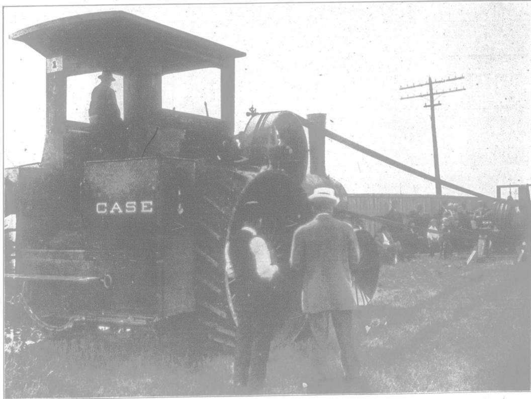
This picture shows the Case 32 horse power simple traction engine under the brake test at the Winnipeg Industrial Exhibition. The brake strength of this engine is from 110 to 125 horse power while its traction power is as rated above. Under the three tests hauling, brake and plowing the above engine was awarded first prize and gold medal by the judges of the motor contest.
