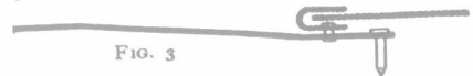
FIG. 3 No. 3 is the old-fashioned cleat shingle now almost entirely driven from the market by the Safe Lock. These do not always shed water, and it is almost impossible to keep them from leaking after they have been on for a season or two.
