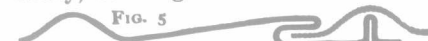
FIG. 5 No. 5 is a side slip pattern, similar to many now on the market. The one shingle slips into the other, but does not lock. Shingles constructed in this way pull apart easily and must not be confused with the positive lock in our Safe Lock Shingles, as shown in Fig. 2.
