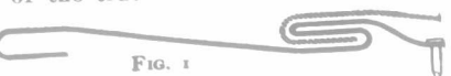
FIG. 1 In Fig. 1 the solid black line shows the top lock, the shaded line the bottom lock. Notice that a
