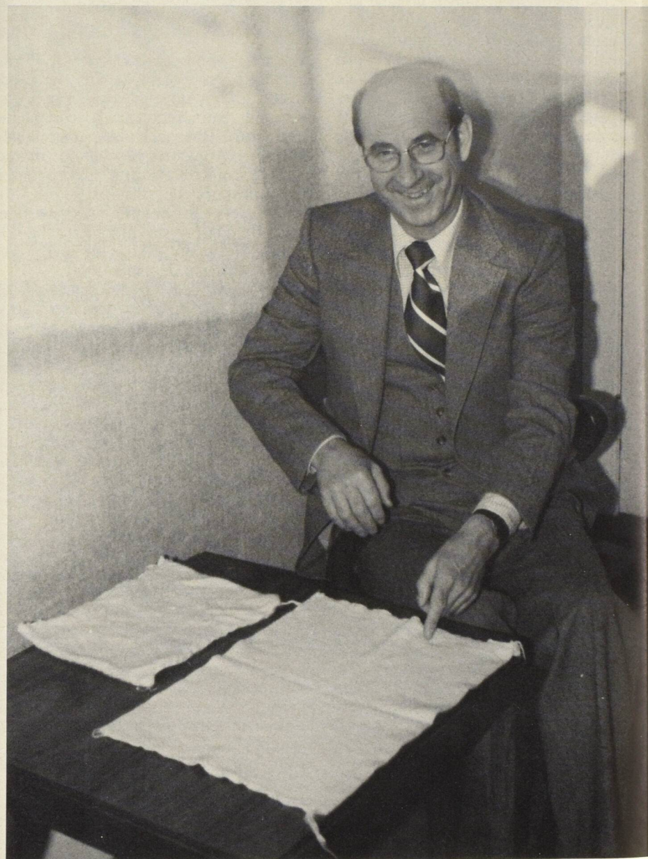
Vice-President Norman Cruickshank shows how Kroy-treated wool sample (right) retains its shape and size while untreated sample (left) shrinks and mats. (Photo: Dr. W.H. Hook)
