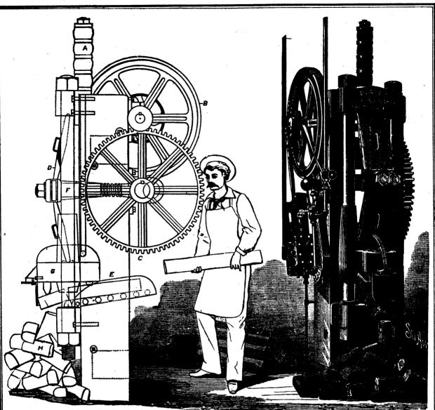
Rubber spring for raising the jaws or knives. Fly-wheel. C.-.Gear-wheel, D.-.Toggie.
