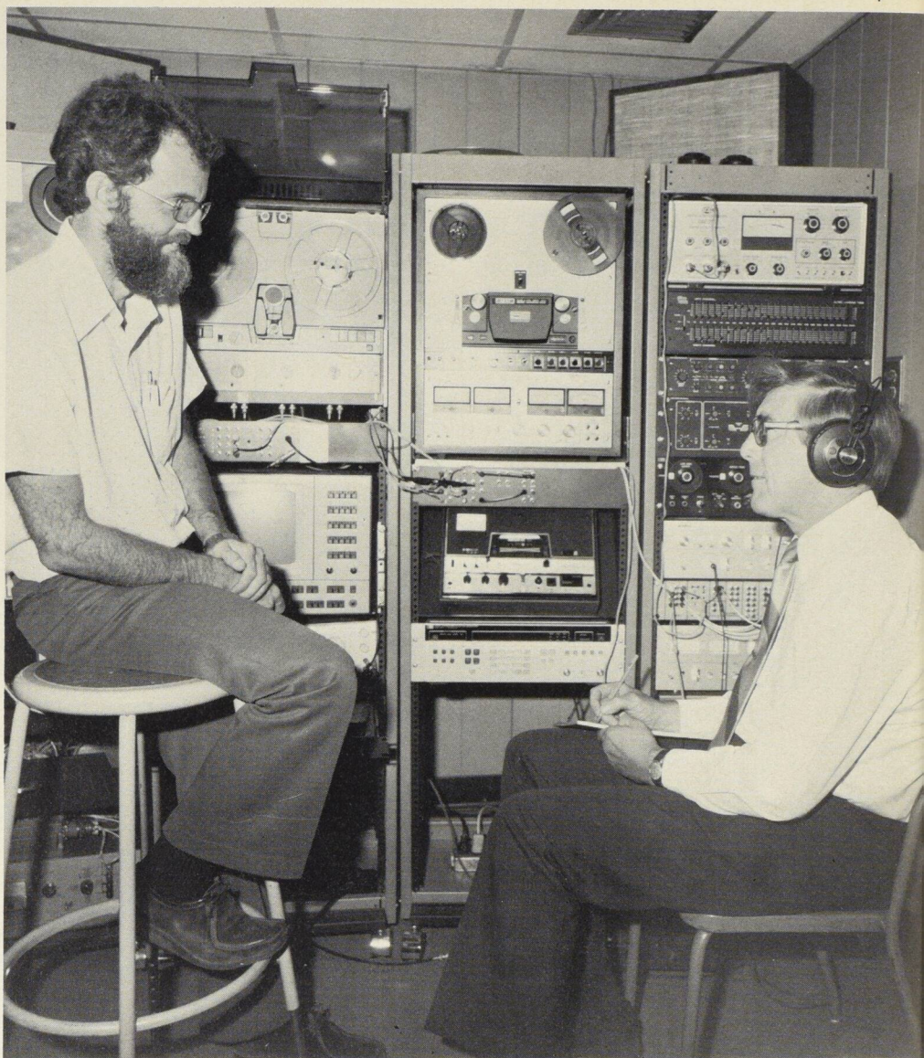
Mike Renton and Bernard Caiger monitor the voice record of an accident flight in the shielded room of the Playback Centre.
