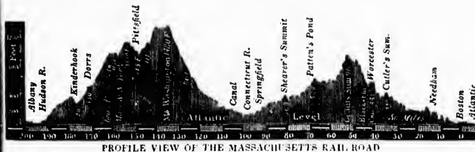
PROFILE VIEW OF THE MASSACHUSETTS RAIL ROAD
