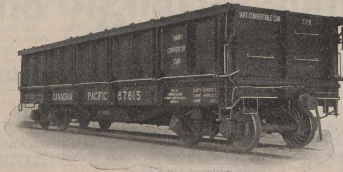
50 Ton Car with Steel Underframe, Steel Stakes, Steel Side Plates and Steel Hopper.
