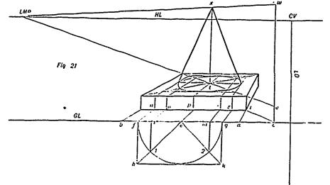
the front edge of the top of the slab, and then towards CV across the top. This is clearly shown in the illustration. The height of both slab and cone is measured on a perpendicular from the point of contact of the near corner of the base of the slab, brought forward in the direction of one of its diagonals from LMP to PP. The line from v to LMP passes through the centre (t) of the base of the cone, and the line from w to LMP passes 6' above it, giving x as the apex of the cone.
