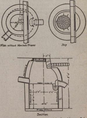
Details of Catch Basins as used in Providence, R.I.
