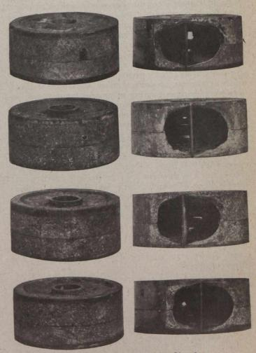
Appearance of Corroded Disc Chambers.
