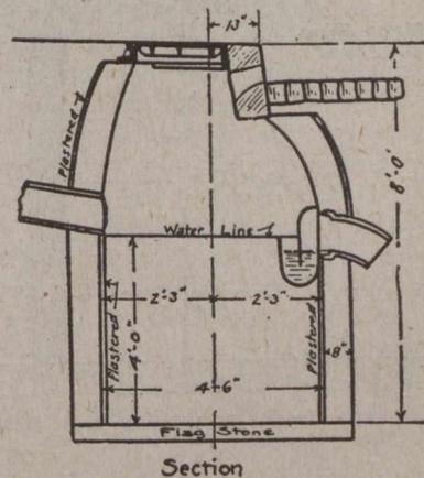
Details of Catch Basins as used in Providence, R.I.
