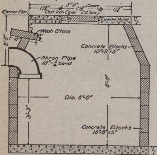
Concrete Block Catch Basins as used in New Bedford.
