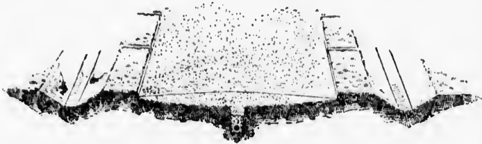
FIGURE 6. A GRAVEL ROADWAY WITH UNDER-DRAIN.
