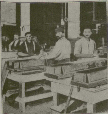
MOULDING COVERING FOR STEAM PIPE.
