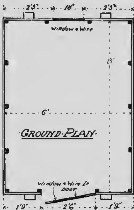
Fig. 33.—Showing ground plan of colony house for growing stock.
