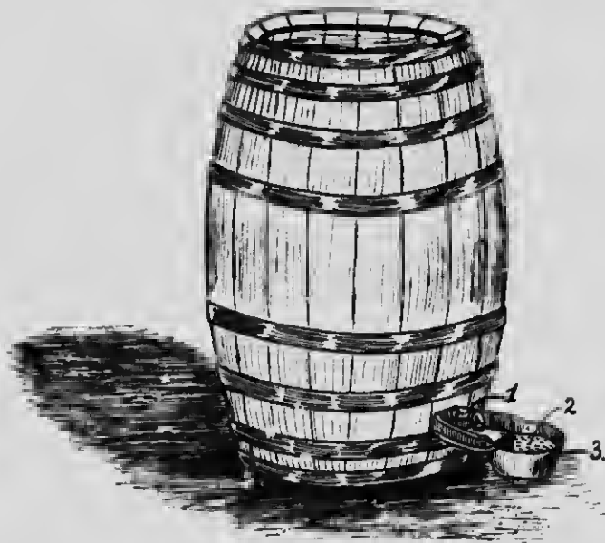
Fig. 44.—A labor-saving device, showing method of providing chicks with a continuous supply of fresh water. The barrel is fitted with a water valve which controls the flow of water. No. 1 is the pipe entering the barrel and fitted with a stop cock. No. 2 is water in the water cup. No. 3. When the water cup is full the weight is sufficient to close the stop cock in the pipe.
