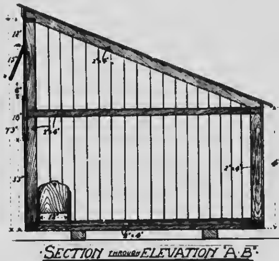
Fig. 38.—Showing side construction of house in Fig. 35.
