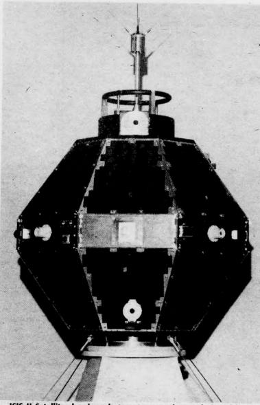
ISIS II Satellite showing photometer experiment designed by Dr. Shepherd at bottom centre. This was used for measuring the auroral intensity and played an important part in the discover of daytime auroras.
