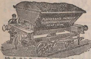
59—R. H.'s Patent 6-Ton Steel Double Side Tip Wagon to work with ordinary tip Wagons
