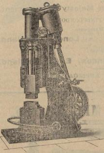
tion 2 to 3 the passage A is gradually closed and therefore some air is forced alternately through the pasages B and C, raising and depressing the hammer piston until when the position 3 is reached, A is entirely closed and all the air is forced into the hammer cylinder, thus producing the maximum blow
