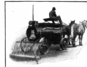
**CASE "Two-in-One" Engine Tender and Sprinkler**
