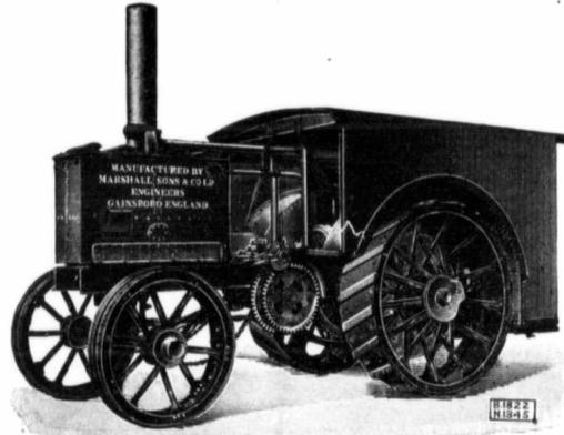
The above represents a 32 H.P. Draw Bar and 60-70 Brake H.P. "CASS" F. Tractor, with two travelling speeds.
