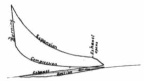
Fig. 157.—Indicator Diagram of Gas Engine, slightly exaggerated
