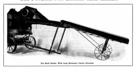
We make independent extra length carriers, which may be attached to the regular carrier, fourteen feet long, with leg support or two-wheel trucks, quickly attached and driven by a sprocket and chain from the upper shaft of the regular carrier. With it attached there is no loss of grain by littering or trampling under foot. It is especially desirable in feeding loose grain in windy weather.
