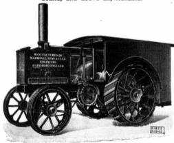
The above represents a 32 H.P. Draw Bar and 60-70 Brake H.P. "CASS" F, Tractor, with two travelling speeds.
