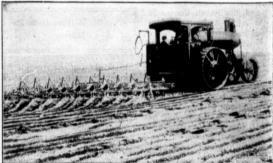
Avery Undermounted Steam Engine and "Self-Lift" Plow.
