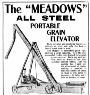
Top and Bottom Sections are both 9 feet long. Middle Sections 4 and 8 feet long. The Sections are coupled together with cast coupling and the Elevator can be easily and quickly taken apart by removing 4 bolts and can be put together just as easily and as quickly. The Capacity is practically unlimited—the greater the speed and Horse Power the greater the capacity. The "Meadows" is positively the
