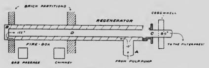
Fig. 6.-Theoretical Working of a Wet-Carbonizing Oven.
