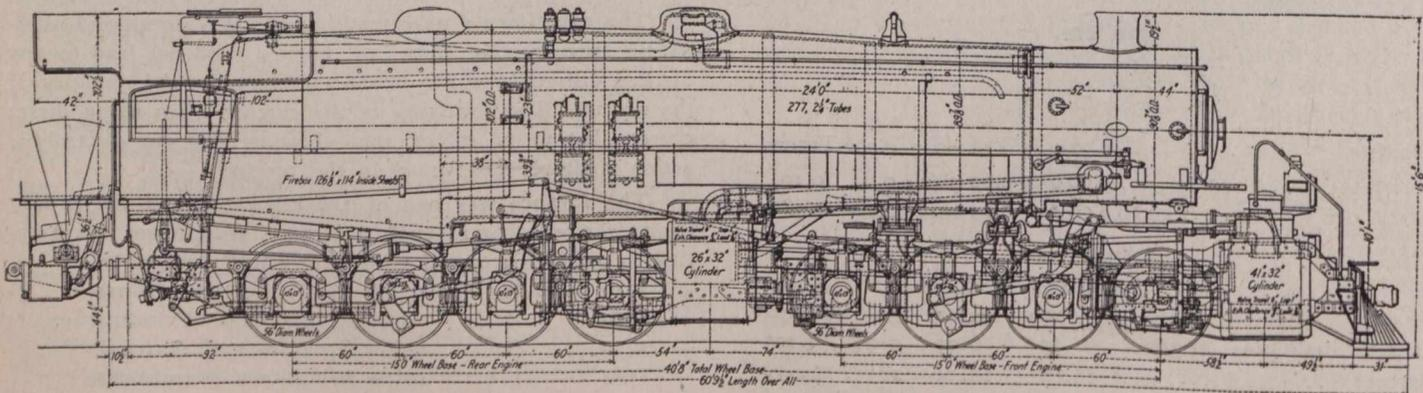
**SIDE ELEVATION AND CROSS SECTIONS OF 230-TON ARTICULATED COMPOUND LOCOMOTIVE**
