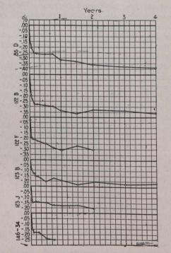
Fig.1. Linear Contraction of Bars of Neat Cement Kept in Air for Four Years, Expressed in Per Cent.
