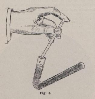
To test for the presence of indol, place 20 c.c. of the water with 50 c.c. of a sterile solution of peptone (10 grammes peptone, 1 litre water) in a test tube and transfer to the incubator for four days at  $38^{\circ}$  to  $40^{\circ}$  C. At this temperature common water bacteria will succumb, but bacteria of the colon group will be encouraged.
