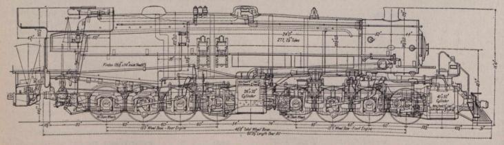
SIDE ELEVATION AND CROSS SECTIONS OF 230-TON ARTICULATED COMPOUND LOCOMOTIVE
