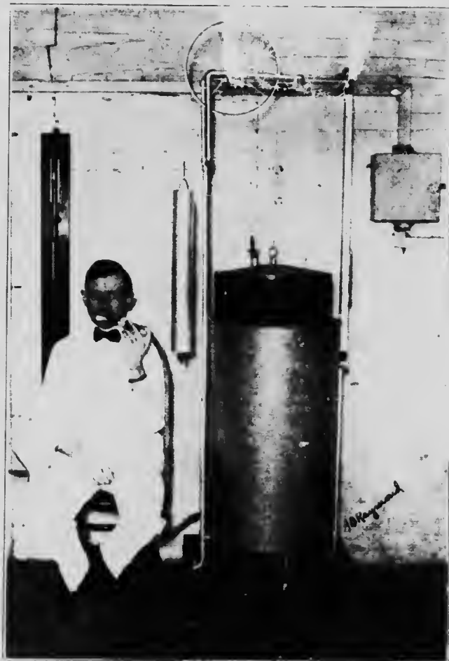
179 The Tissot spirometer. In actual experiment, subject is reclining or lying down and the valves and mouthpiece are held with a clamp.
