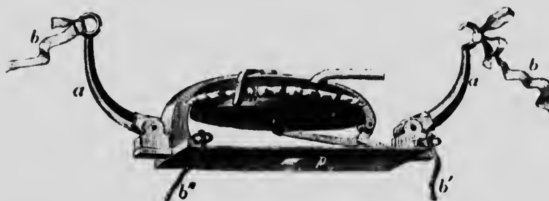
FIG. 108. Pneumograph. The straps (b, b) are held around the thorax, and the tube of the tambour connected by rubber tubing with a recording tambour.
