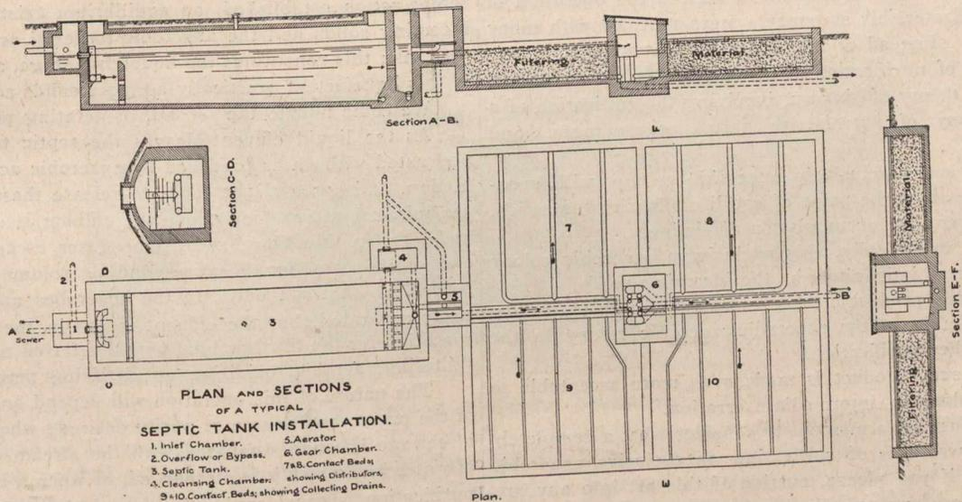
Fig. 1.—Plan and Sections of Typical Septic Tank System.
