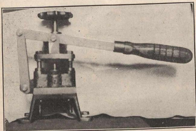
Fig. 3.—Bullet-sizer and Lubricator.
