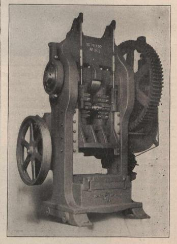
Fig. 5. The Trimming Press.
