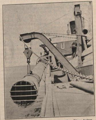
Fig. 3.—" Galveston," showing Suction Pipes being lowered over side.
