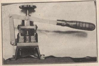
Fig. 3.-Bullet-sizer and Lubricator.
