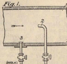
otherwise, a certain pressure, known as velocity pressure, is set up in the Pitot tube, because some of the momentum of the impinging air is destroyed by the quiescent air in the tube. It has been shown by Lord Rayleigh and confirmed
