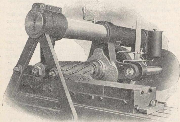
Evidently a large amount of work that engine builders and general machinists are now planing or shaping can be done on a miller at the above rate.
