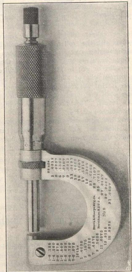
nut. This is a valuable feature when measuring a number of pieces for comparison as sufficient tension can be put on the spindle to prevent its turning when the work is passed between the measuring points, and at the same time the spindle can be left sufficiently free to allow of slight adjust-
