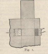
ments. When the clamping ring has been set to exert a certain tension, the rotation of the spindle cannot alter the setting of the tension for the reason that the clamping ring is held stationary and forms part of the bearing for the spindle. Referring to the cuts, figures I, 2, 3, and 4, the operation of the mechanism is as follows: The split clamp ring 2, figure 2, fits the measuring spindle with a sliding fit when open, thus measuring a longer bearing for the spindle than
