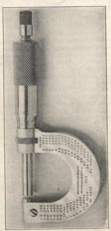
nut. This is a valuable feature when measuring a number of pieces for comparison as sufficient tension can be put on the spindle to prevent its turning when the work is passed between the measuring points, and at the same time the spindle can be left sufficiently free to allow of slight adjust-
