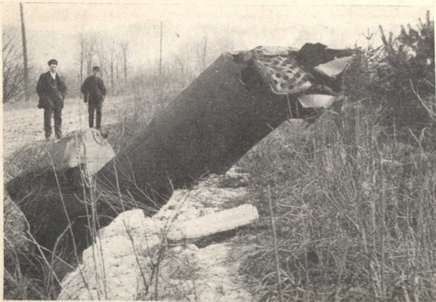
Shell of Saw-mill Boiler, carried nearly a quarter of a mile and skipping like a stone
