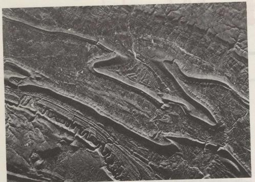
Star-1 image of terrain in the eastern United States shows subtle relief and geologic structure illustrating the advanced resolution and image quality of the system.
