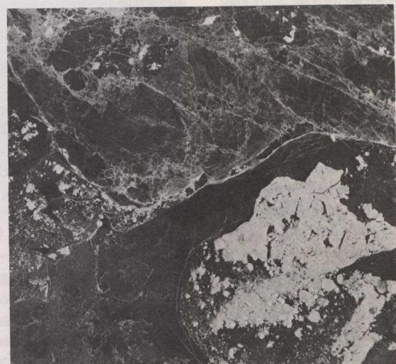
Star-1 synthetic aperture radar image of ice fields in the Beaufort Sea made from more than 9 000 metres above and transmitted to a ground station by digital data downlink shows ice types, small multi-year ice hazards, pressure ridges, ice breaker tracks and drilling vessels.
