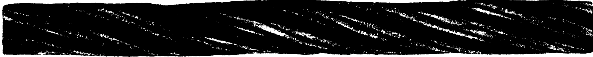
Illustration of \frac{3}{4} " diam. Special Improved Patent Steel Wire Rope, 1760 yards long, supplied to Dalzell Colliery, Motherwell, Scot., which ran two years and 8 months, shewing condition when taken off. Previous rope from another maker lasted 1 year and 9 months
