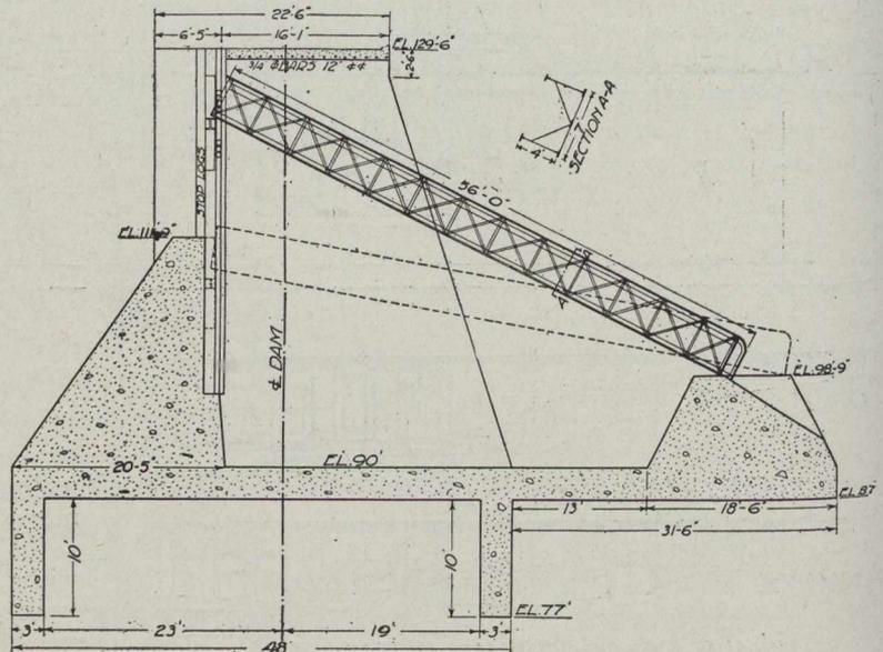
Section D-D Through Log Sluice.
