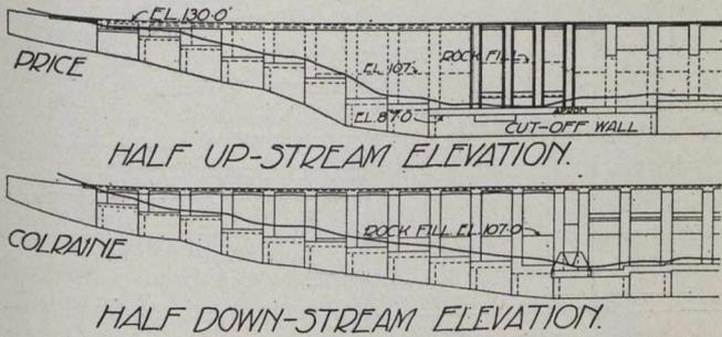
On the down-stream side of the deck slab and resting on the floor, the design calls for a stone embankment with a slope of 1:1, the exposed side to be faced with cement mortar.
