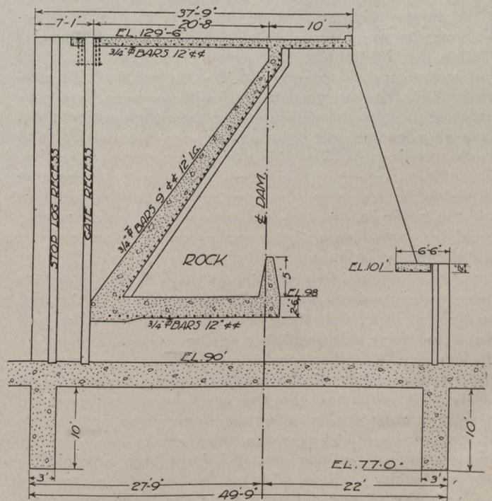
Section B-B Through Sluices.
