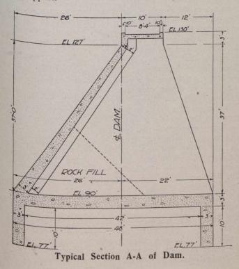
on the floor, the design calls for a stone embankment with a slope of 1:1, the exposed side to be faced with cement
