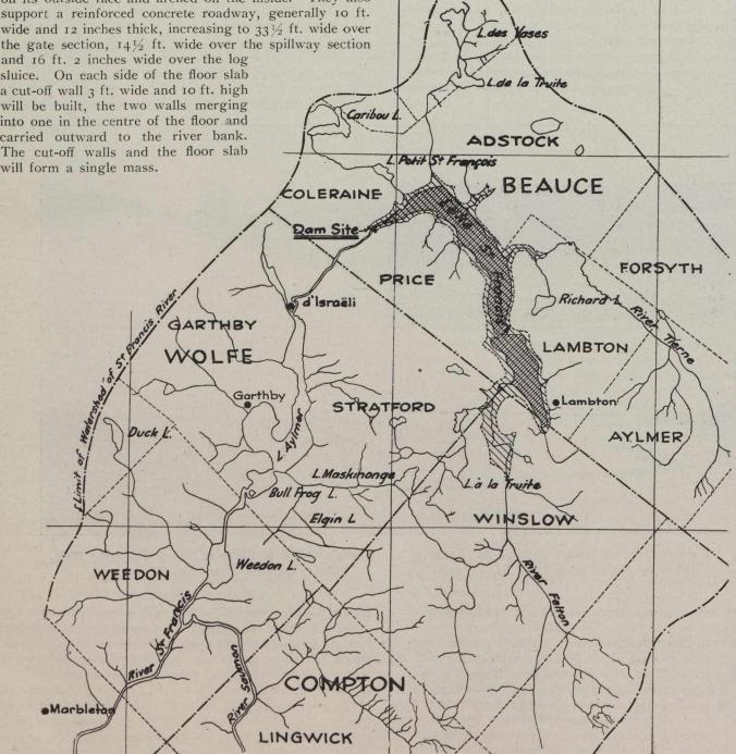
St. Francis Drainage Area, Showing Present Area of Lake (El. 100.00) Shaded Heavy; Land Flooded When Level is Raised (El. 127.00) Shaded Light.
