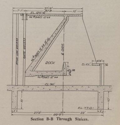
The bed of the river at the site of the dam is composed of a very stiff mixture of clay, small boulders and gravel, into which the whole of the floor slab and the cutoff wall are to be embedded. The river will be diverted by cutting a new channel and by cofferdams, and the river bed excavated, for the foundation of the main dam and aprons, to hard pan about 2 ft. below the natural
