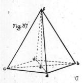
raise a vertical line—that is, a line parallel to the sides of the paper, not a line perpendicular to any of the lines in the base. Compare the distance c b with that from b to f, and complete the solid by drawing lines from f to the four corners of the base, the back lines, of course, not showing in the finished drawing.
