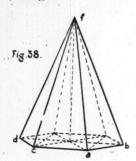
following the directions given for drawing the hexagon, these points will help to correct one another. After completing the hexagon, raise a perpendicular (as before, parallel to the sides of the paper) from the point where the diagonals of the hexagon cross one another, and on this mark off the point f by comparing d b with b f. All that remains is to join the apex to the points of the hexagon.
