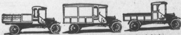
Three of the many body styles that may be mounted on the Ford truck chassis
