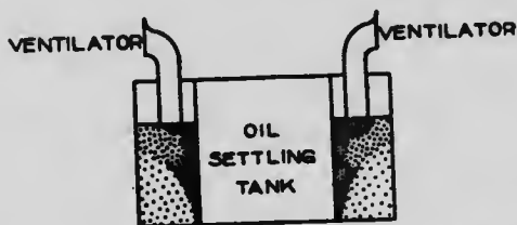
Fig. 19. Section through heating wheat near stokehold bulkhead.
