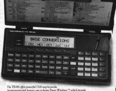
The T1-95 offers powerful /200-step keystroke programming and features our exclusive Power Windows,™ which provide easy access to the functions and flexible file management system.
