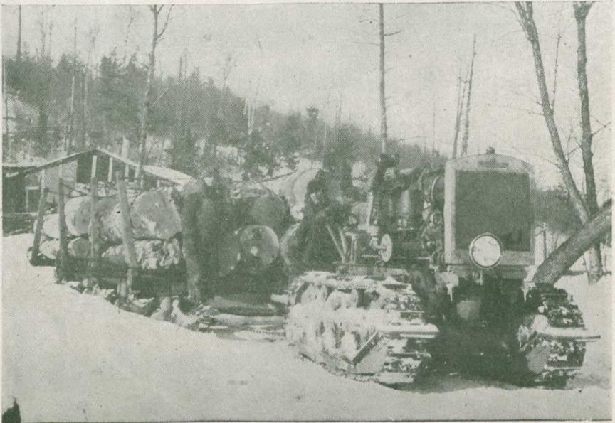
Picture of Monarch Tractor Pulling Load of Logs Through Heavy Snow in Lumber Camp
