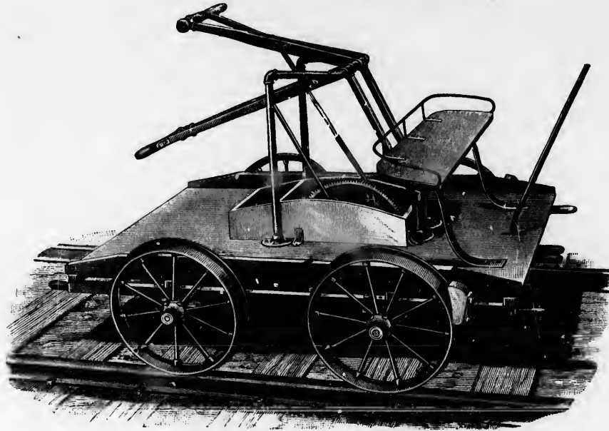
Frames of all Cars made of selected White Oak. Capacity of above Car, two to four operators and three inspectors. Geared 3\frac{1}{2} to 1. Weight, 550 lbs. Price, single car, $60.00.
