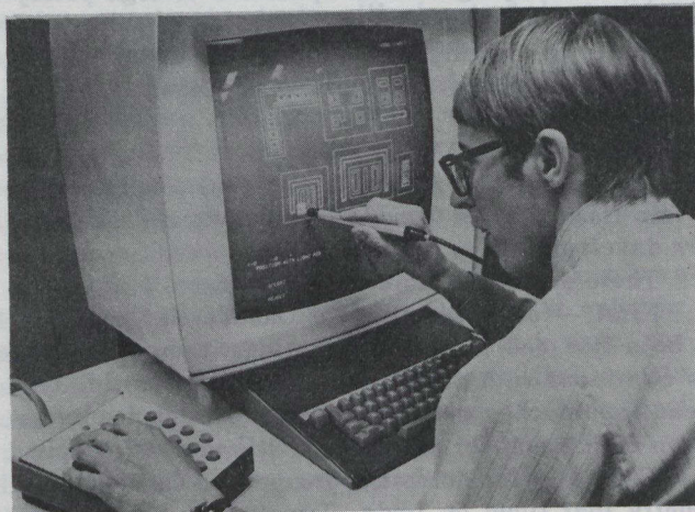
Computer application engineer Chris Morris zeroes in on one component of a new integrated circuit design, using light pen and special keyboards of a display unit linked to an IBM 360/67 computer.
