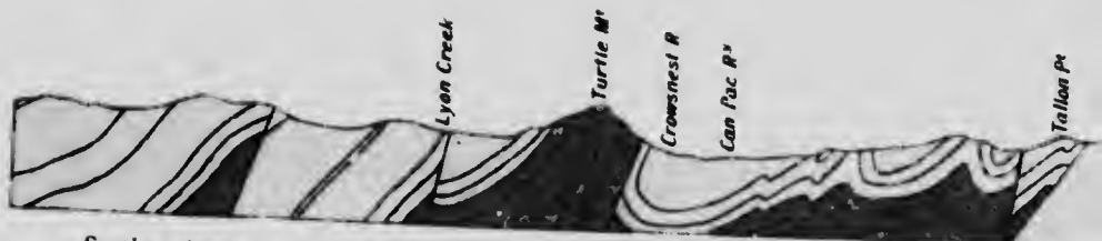
Section along Canadian Pacific Railway near Frank, Alberta. Scale, 2 miles to 1 inch (After W. W. Leach)
