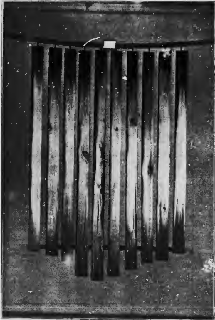
Penetration obtained in jack pine heartwood using a half-hour pressure period (about one-twelfth actual size). See Table 2.
